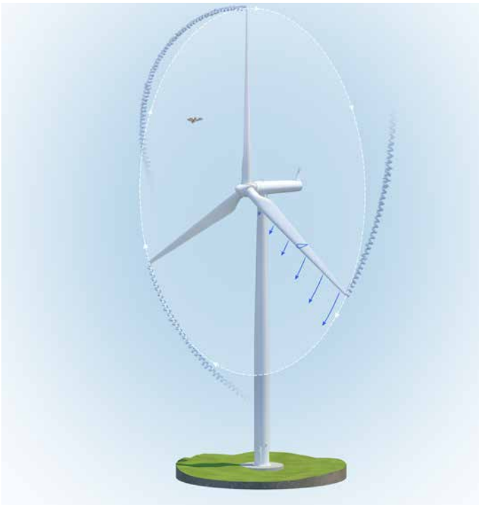
Figure 1. Low-pressure regions on the downwind side of the blade and high-pressure regions on the upwind (blade surface) side are caused by local flow accelerations. Vortices also form downwind from the blade tip. These can cause barotrauma in bats. Graphic from Lawson et al. 2010. An Investigation Into the Potential for Wind Turbines To Cause Barotrauma in Bats. PLoS ONE 15(12): e0242485.
