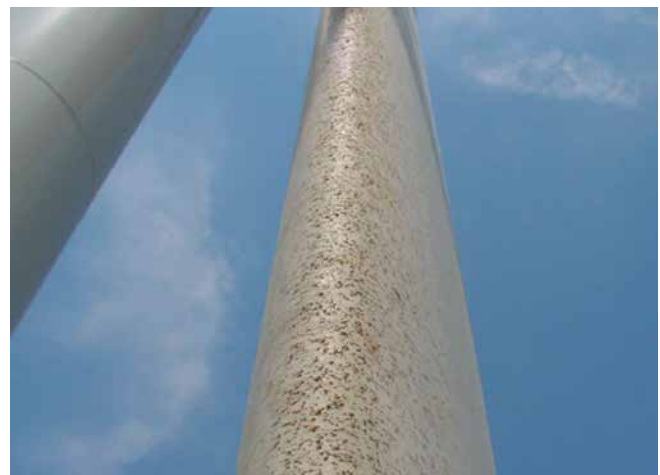
Figure 7.3. Image of turbine blade leading edge with evidence of invertebrate body parts. Image from Voigt [4].
