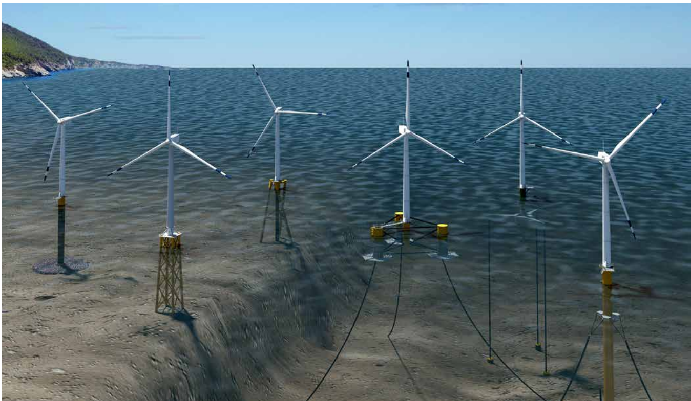
Figure 1.2. Offshore wind foundation types for fixed-bottom turbines (three turbines on left) and floating wind turbines (three turbines on right). Illustration by Josh Bauer, National Renewable Energy Laboratory.
