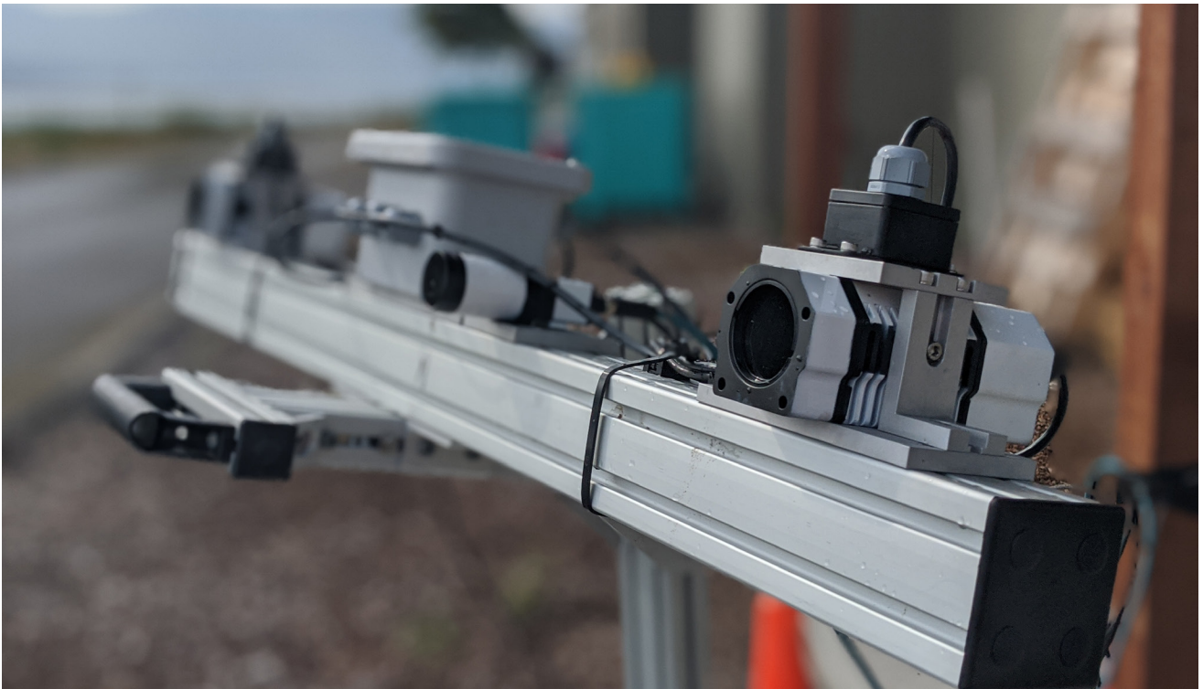
Figure 5. ThermalTracker camera system for monitoring bats and birds at wind farms. Photo from Pacific Northwest National Laboratory.
