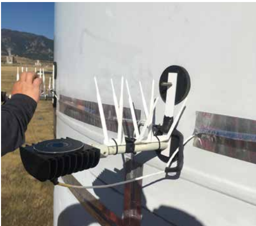
Figure 3. UV illuminator unit magnetically attached to wind turbine monopole. Photo from Paul Cryan, USGS
