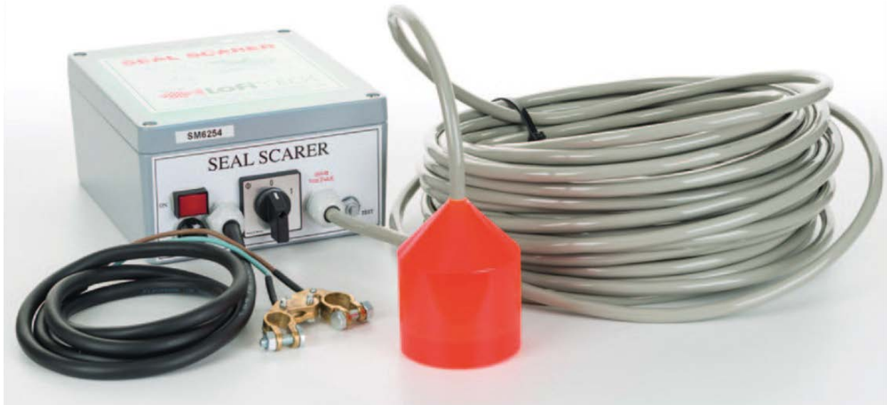
Figure 2. Lofitech Acoustic Deterrent Device of the type used during the construction of the Belwind wind farm. The figure shows the control unit (left) and transducer (on the right). The control unit contains a pulse generator and an amplifier and transmits random bursts of audio frequency signals to the transducer, where they are converted into intense sound (from www.seiche.com).
