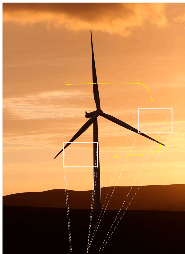
Figure 2. Example thermal-imaging camera frame views (white squares) from nocturnal survey station as views shifted while slowly swiveling camera mounted on tripod. During actual surveys, the sky was completely dark.
