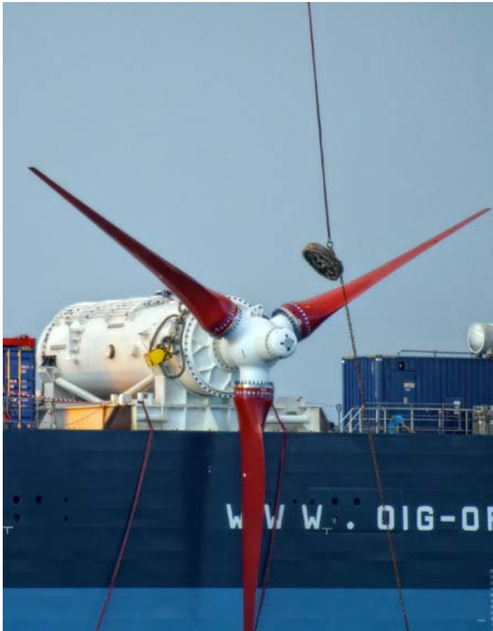
Living up to promise: Andritz Hydro Hammerfest's 1MW HS-1000 turbine has hit rated capacity during Orkney sea trials
