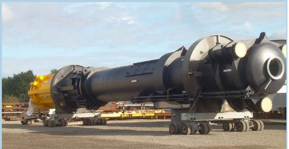
Local content: major steel components for OPT's first US-made PB150 will be incorporated with power take-off by Vigor Industrial in Portland shipyard ahead of installation off Reedsport by early 2013
