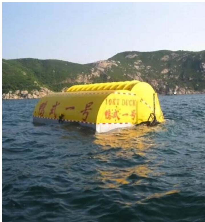
'Floating duck': the 10kW Guangzhou device is one of the myriad technologies being pursued by Chinese research institutions
