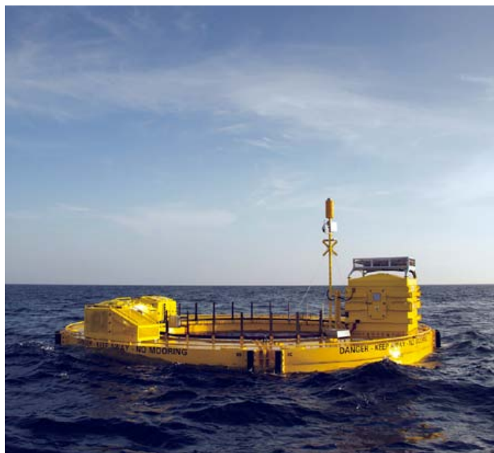
Ring of confidence: Fred Olsen became one of the few to install a wave energy converter in English waters earlier this year with the deployment of its Bolt Lifesaver
