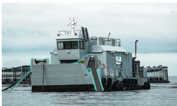
Carnegie's MoorPower wave converter system (image courtesy of Carnegie Clean Energy).
