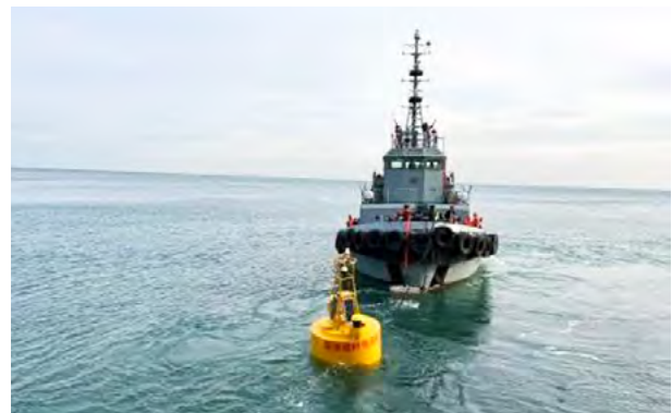
wave energy - solar energy ocean buoy in sea trial operation
