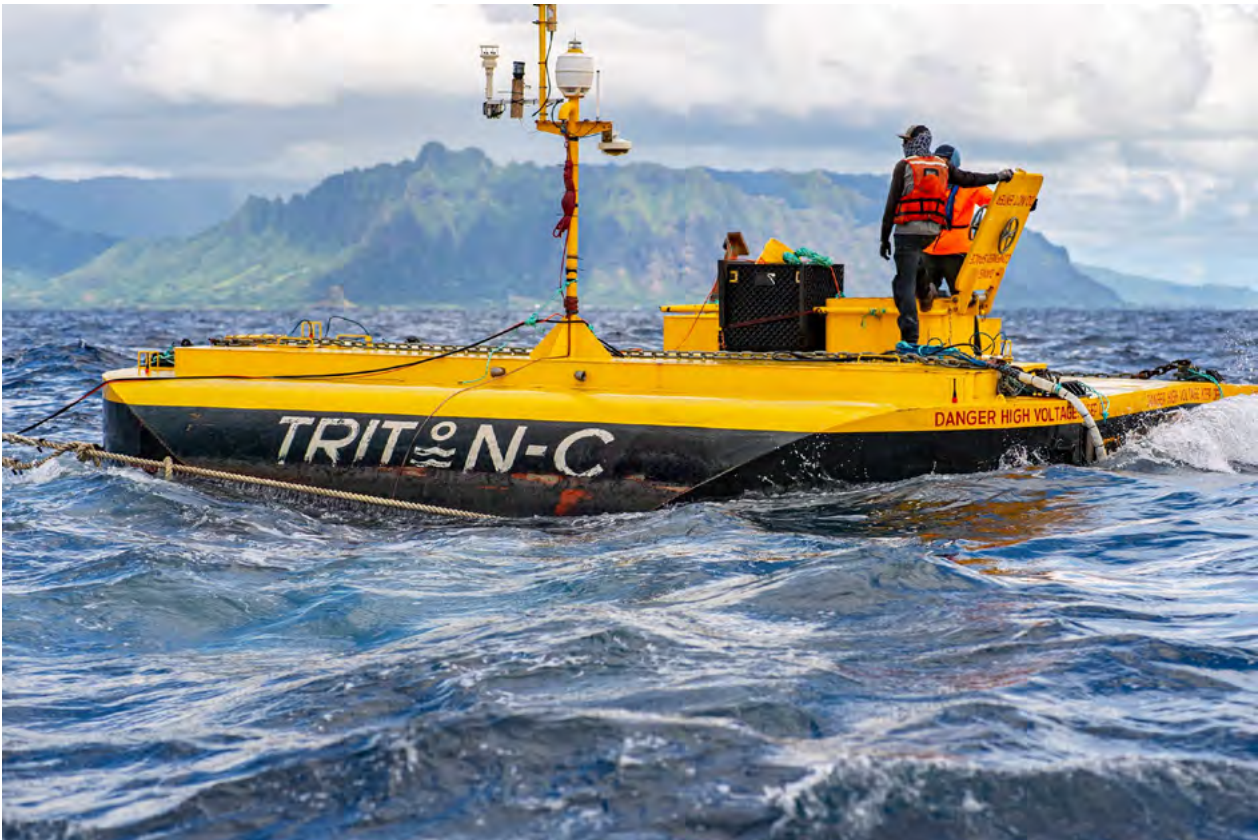
Oscilla's Triton-C wave energy device is towed to the grid connection point at the Wave Energy Test Site in Hawaii. Source: Oscilla Power, Inc.
