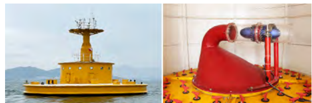
OWC ocean buoy in sea trial operation
