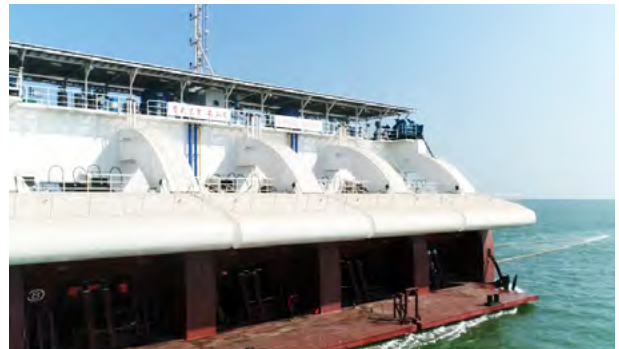
500 kW “Zhoushan” “Changshan” WEC devices
