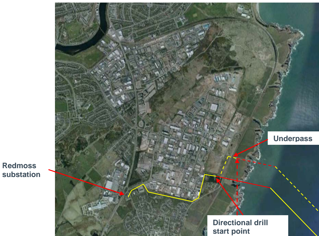
Figure 4-4 Cable route 2 with two options for directional drill locations (only one to be used) and expected length of directional drill (red line).
