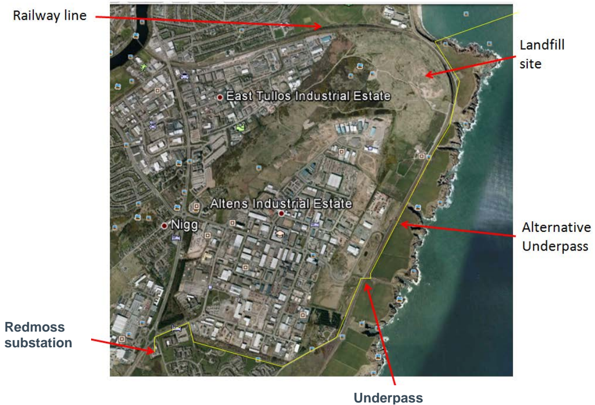
Figure 4-4 Cable route 2 with two options for directional drill locations (only one to be used) and expected length of directional drill (red line).
