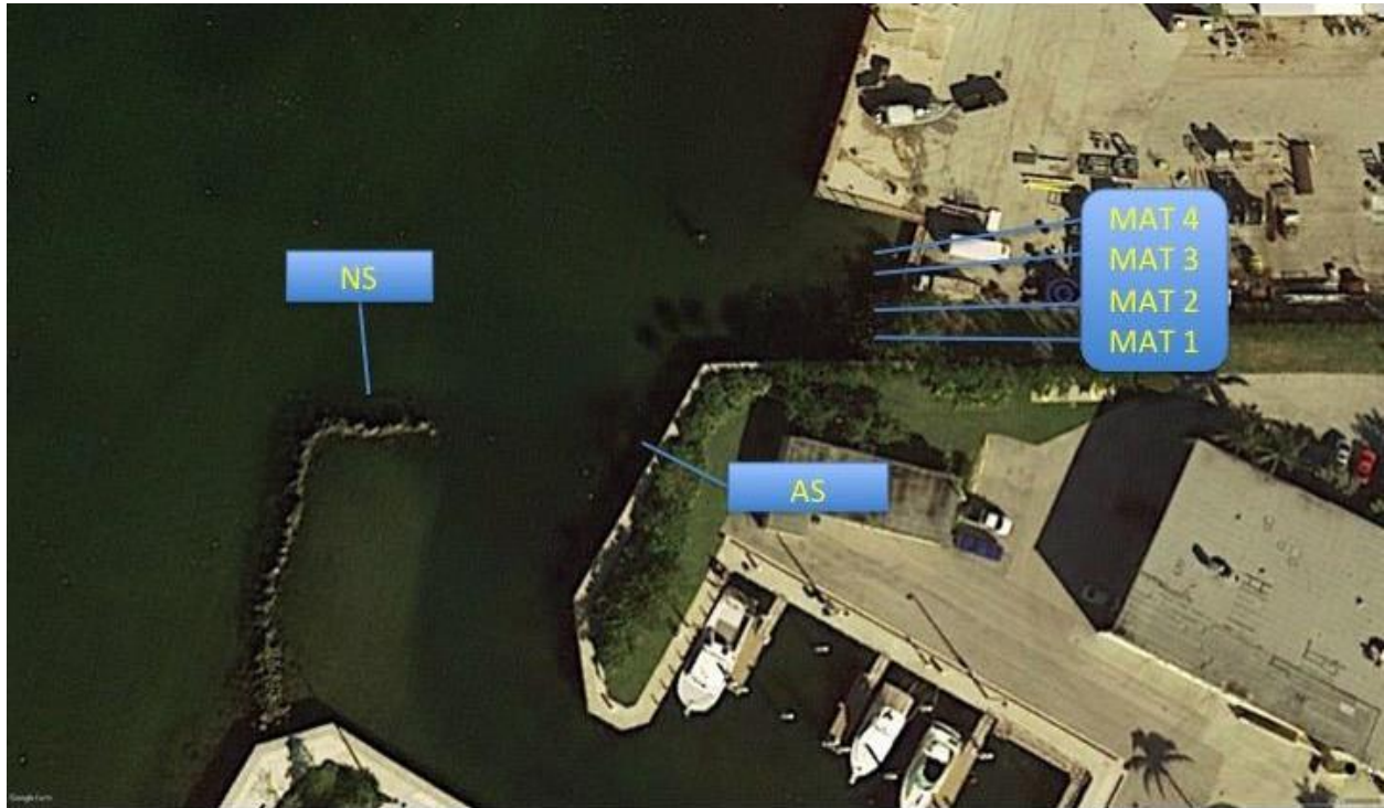
(Fig. 4) Satellite Map of the different study sites. Each MAT is composed of ECONcrete® Bio-Enhanced units and control units. The locations are MAT 1 (M1E, M1C), MAT 2 (M2E, M2C), MAT 3 (M3E, M3C), MAT 4 (M4E, M4C), limestone boulders water breaker (NS), and construction site remnants (AS).
