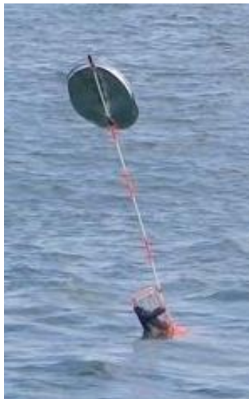
Figure 4.7. Spar buoy with GPS and radar deflector drifting over the instrument platform (lander). IcTalk speaker unit is drifting 2 m below the surface.
