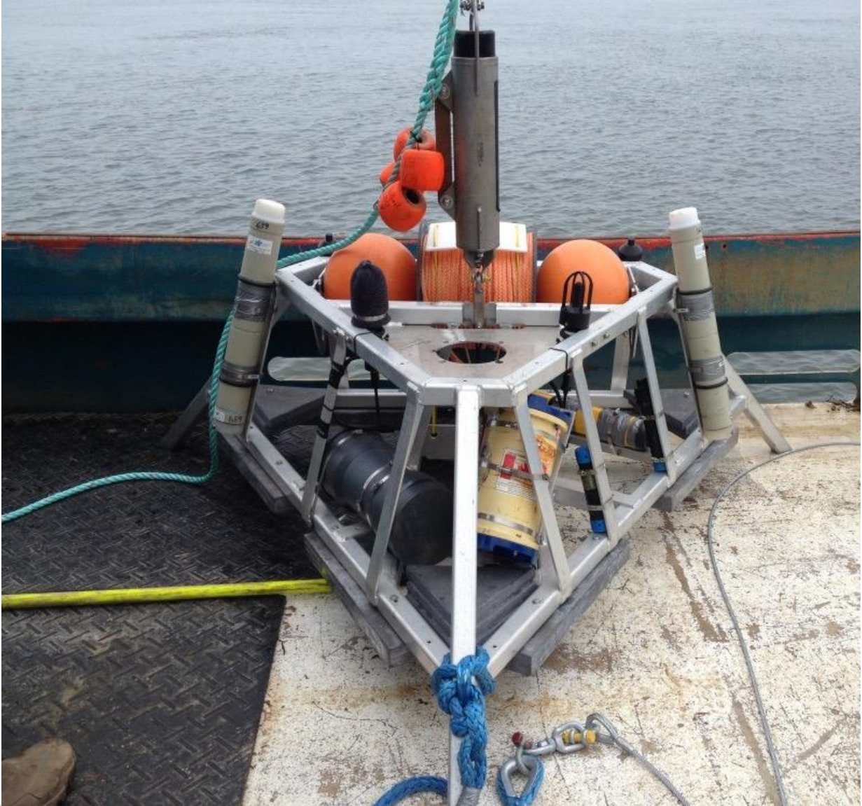
Figure 4.2. Image of instrument platform prior to deployment. Note the 2 C-PODs in the far corners and the shrouded and non-shrouded icListenHF hydrophones (black sensors) located above their battery packs. The instrument hanging vertically above the frame is the Teledyne Benthos 866-a acoustic release.
