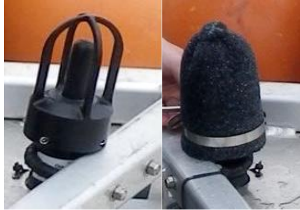
Figure 3.2. IcListenHF hydrophone tip with custom made HDPE guard (left) and with 0.5 inch, 20 ppi foam cover secured over the guard (right).
