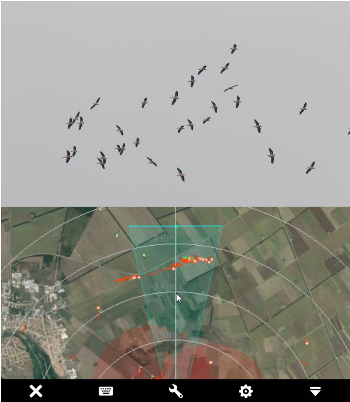
Figure 3. A flock of White pelicans: an illustration of the simultaneous records obtained by every ornithologist in real time, information from Robin Radar System and visual observations.
