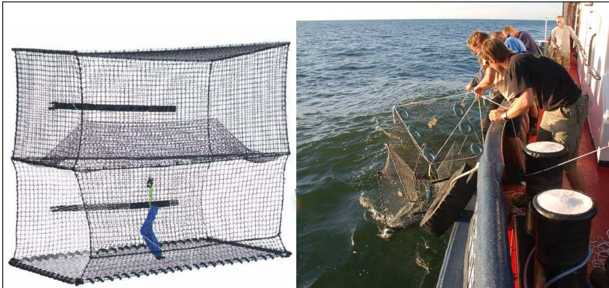
Figure 4. Baited life traps selected for catching cod directly around the wind turbines: bait will be placed in the blue socket. Weights will be attached to the bottom of the trap and buoyancy will be added to the top of the trap.
