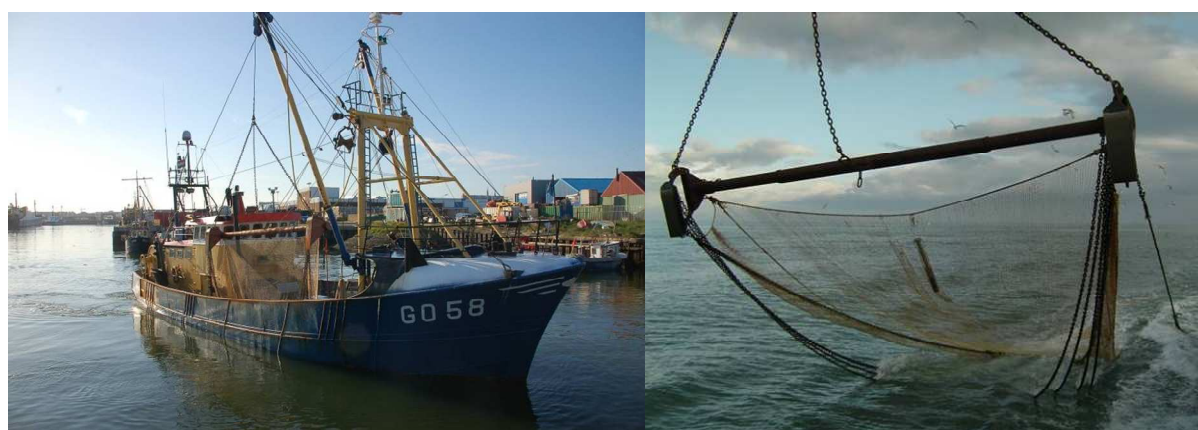
Photo 2. The beam trawler G058 (left, Erwin Winter) and the 6-m beam trawl (right, Olvin van Keeken) that was used for the tagging experiments with sole.
