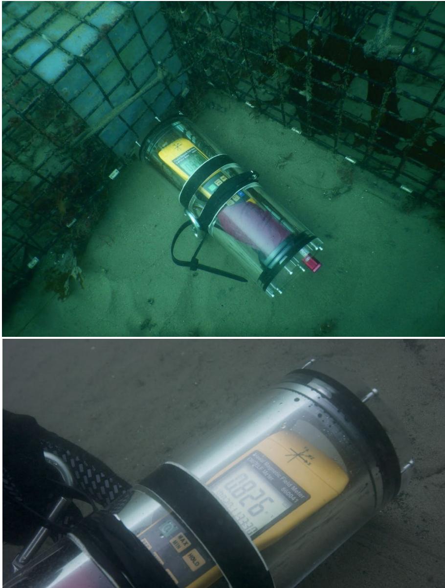
Figure 7. Sper Scientific EMF meter inside the Blue Robotics waterproof enclosure.
