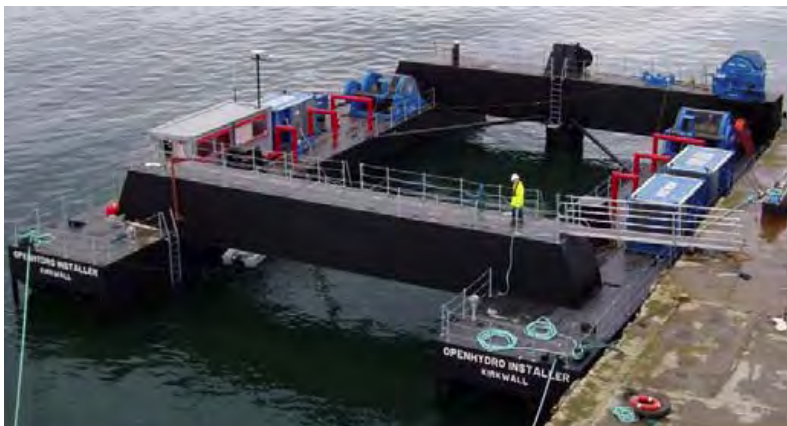
Figure 3.5 OpenHydro’s Deployment Barge, ‘Openhydro Installer’
