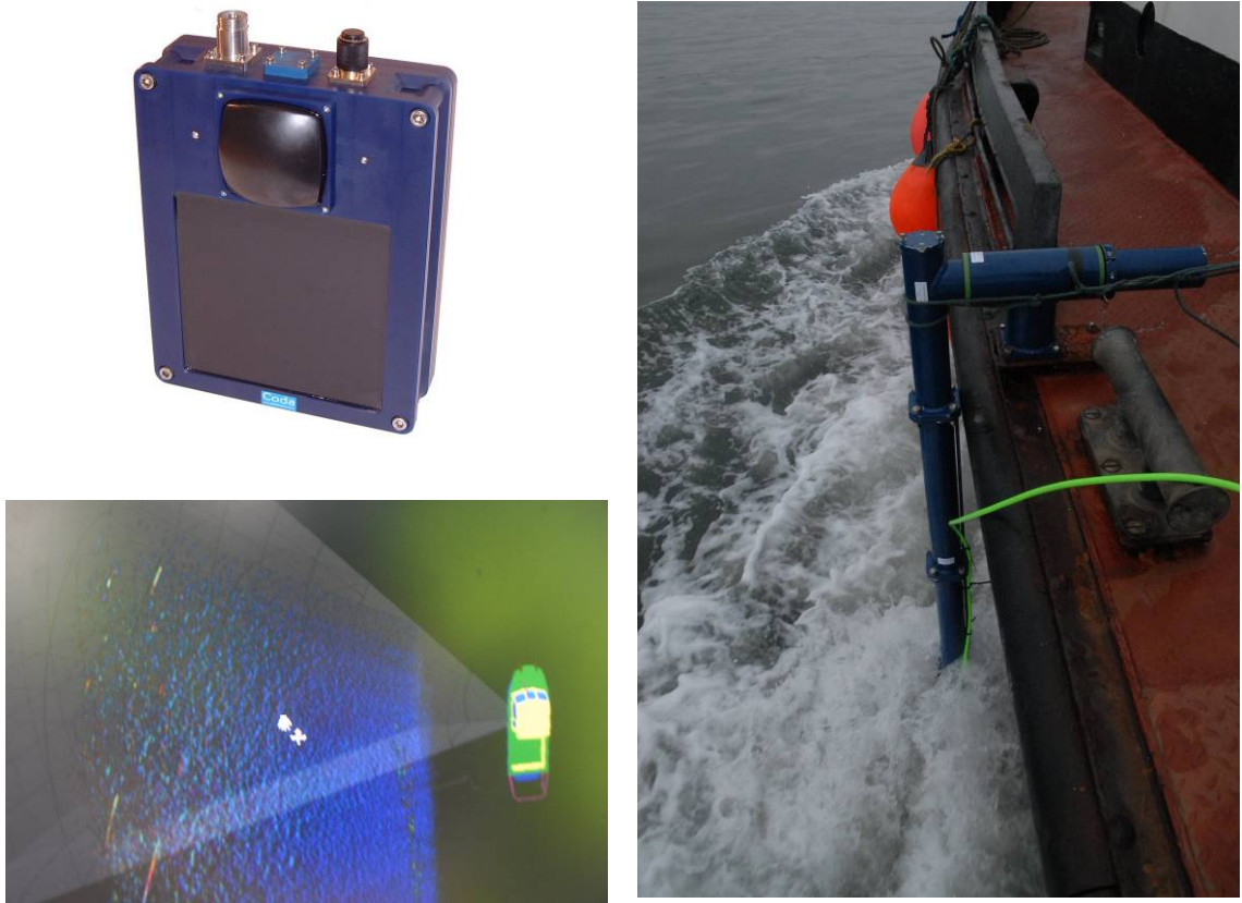
Plate 7-1 the Echoscope™ (top left); the Echoscope™ mounted over the side of the Forth Conserver; and an example of Echoscope™ output (image courtesy of CodaOctopus).
