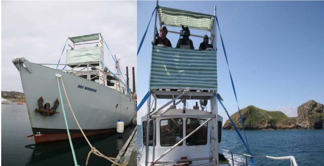
Figure 3-1 Left panel: Boy Brendan , showing sonar bow mount on starboard bow and the scaffolding viewing platform.
