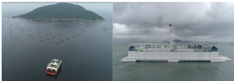
Figure 7. Penghu semi-submersible wave energy aquaculture platform [5].
