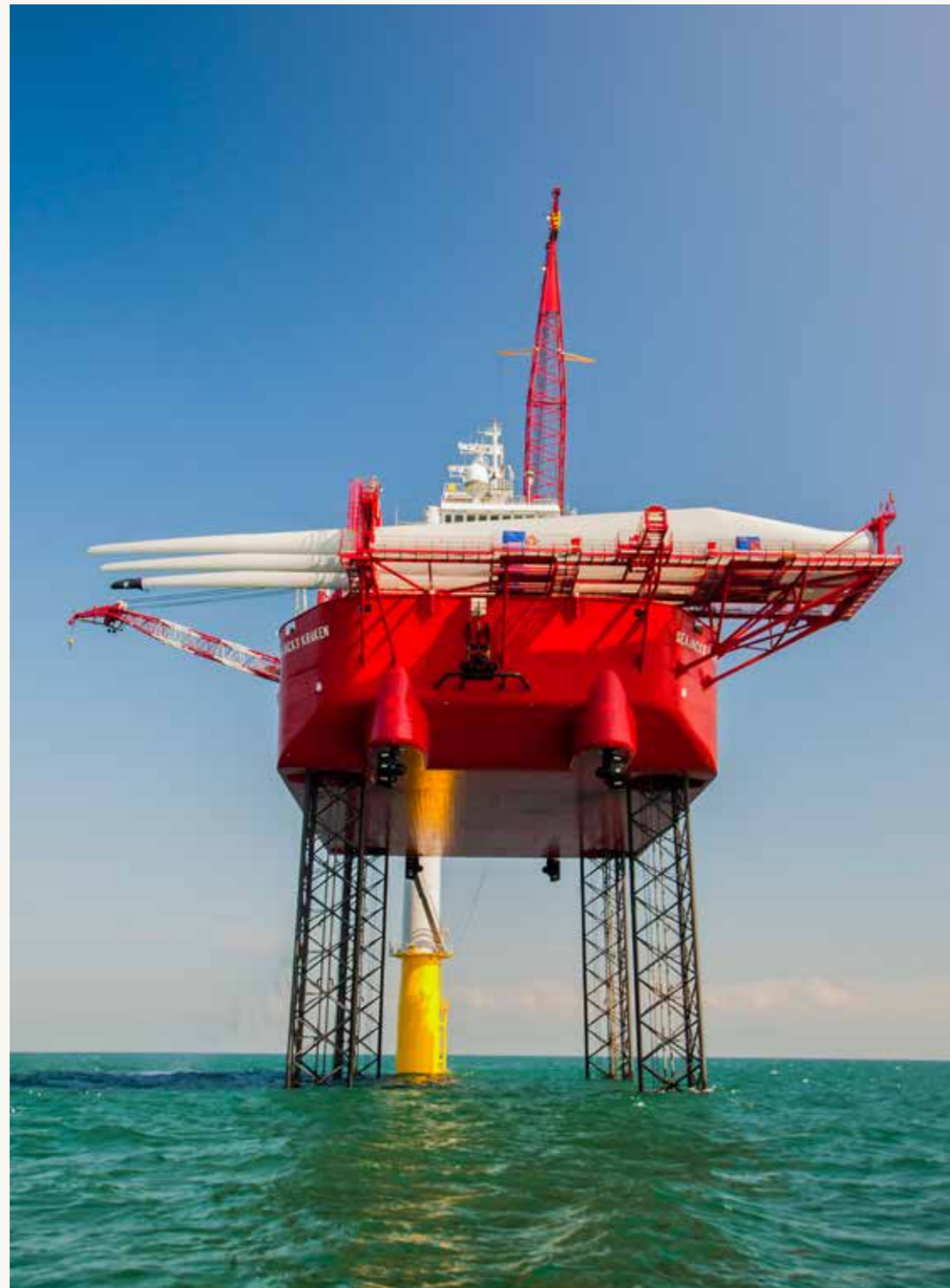
The Krakken, a jack up barge, that is constructing the wind turbines of the Walney offshore windfarm. The farm consists of 102, 3.6 MW turbines, giving a total capacity of the Walney project of 367.2 MW, enough to power 320,000 homes. The rotor diameter of the turbines is 107m for Walney 1 and 120 m for Walney 2. The wind farm is owned and constructed by Dong Energy. Cumbria, UK.
