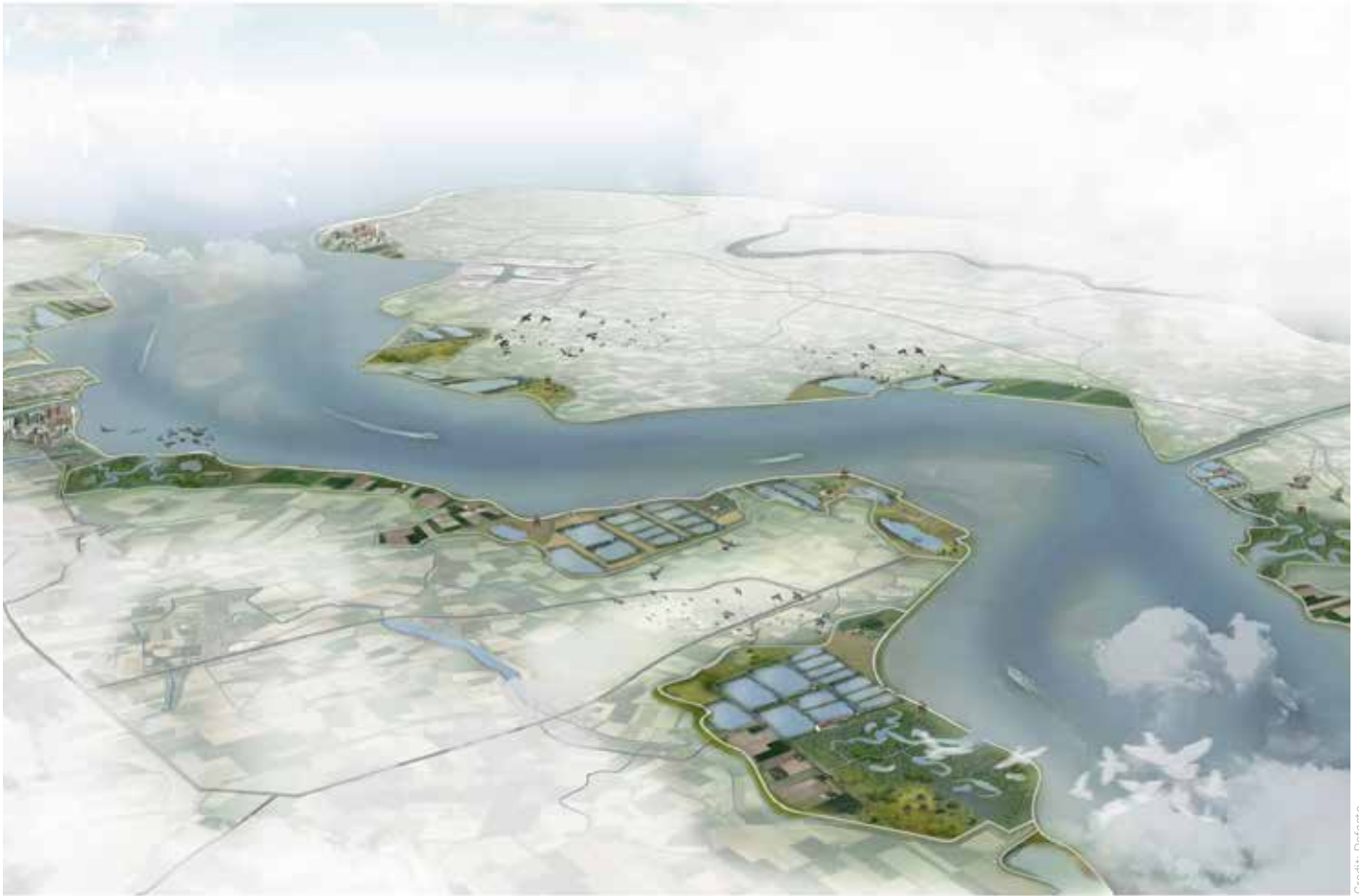
Double dykes with transitional polders are examples of hybrid solutions to coastal protection.
