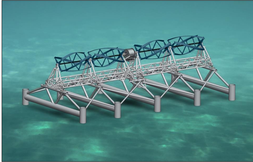
Figure 2.1. Pilot tidal energy device. Drawing of Ocean Renewable Power Company's TidGen™ Power System, the pilot project to be installed in outer Cobscook Bay.
