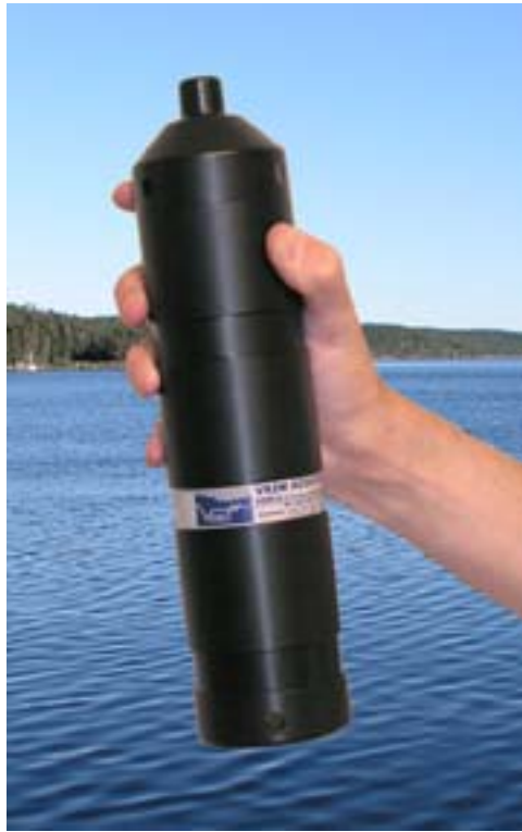
Figure 6-2. VEMCO VR2W Hydrophone Receiver
