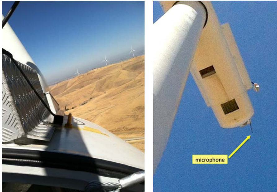
Figure 4. Configuration of nacelle mounted microphones at Vasco Winds Area. A boom mounted from the top of the nacelle extended out and down to place the microphone in the lee side of the nacelle (left). As bats tend to forage in the lee side of natural structures such as trees and cliffs, the directional microphone was positioned to listen outward from the lee side of the nacelle. This also minimized recording distorting sound from the wind and turbine operation.
