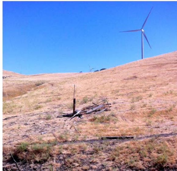
Figure 6. Setting and mounting arrangement of microphone at Turbine 19 ground station at Vasco Winds Area. Turbine 19 can be seen upslope above the station.
