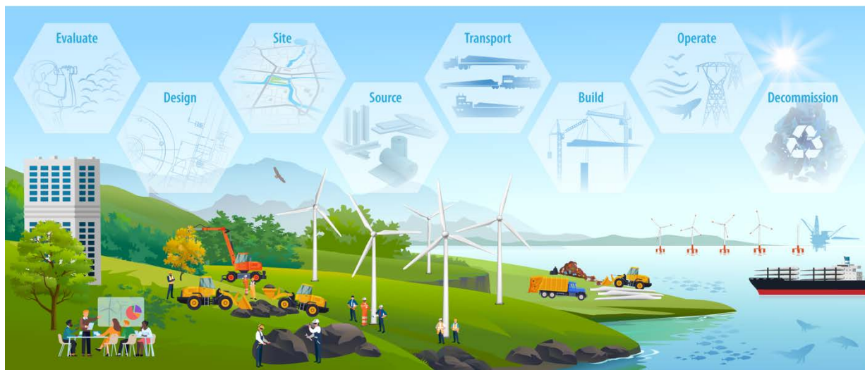
Figure 10. Opportunities for mitigating environmental impacts occur at each stage of the wind turbine and wind plant life cycle. Illustration by AI Hicks, NREL
