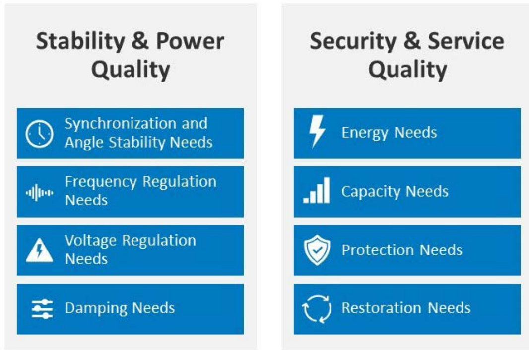
Figure 7. System needs and services of the next generation of wind plants. Adapted from Holttinen and Cutululis, to be published
