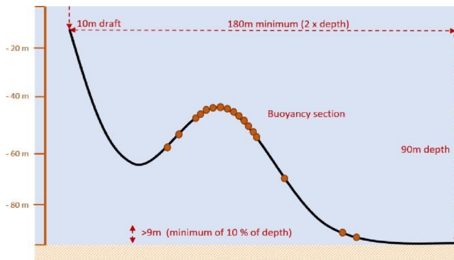
Figure 3-10. CADEMO SATH "Lazy Wave" Cable Configuration
