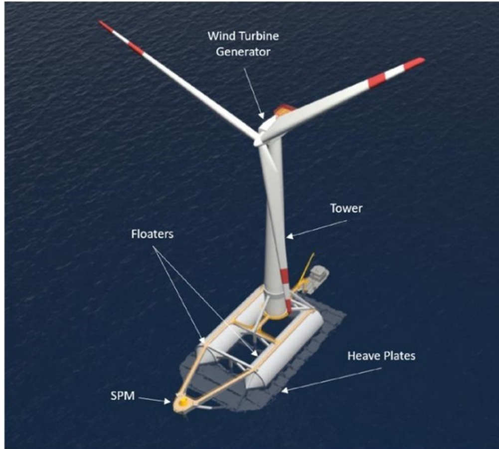
Figure 3-4. CADEMO SATH Floating Barge Technology General Layout
