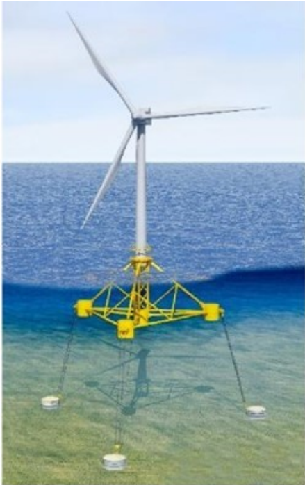
Figure 3-5. CADEMO Offshore Wind Floater Using TLP Technology
