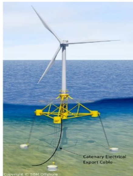
Figure 3-9. CADEMO SBM Offshore Wind Floater Mooring Configuration
