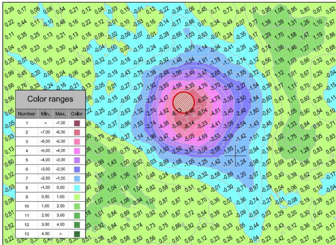
Figure 7: Differential bathymetry map between February 8<sup>th</sup>, 2010 and the reference situation, measured in August 2009. Monopile F03 in the Belwind wind farm (from: Belwind, 2010).
