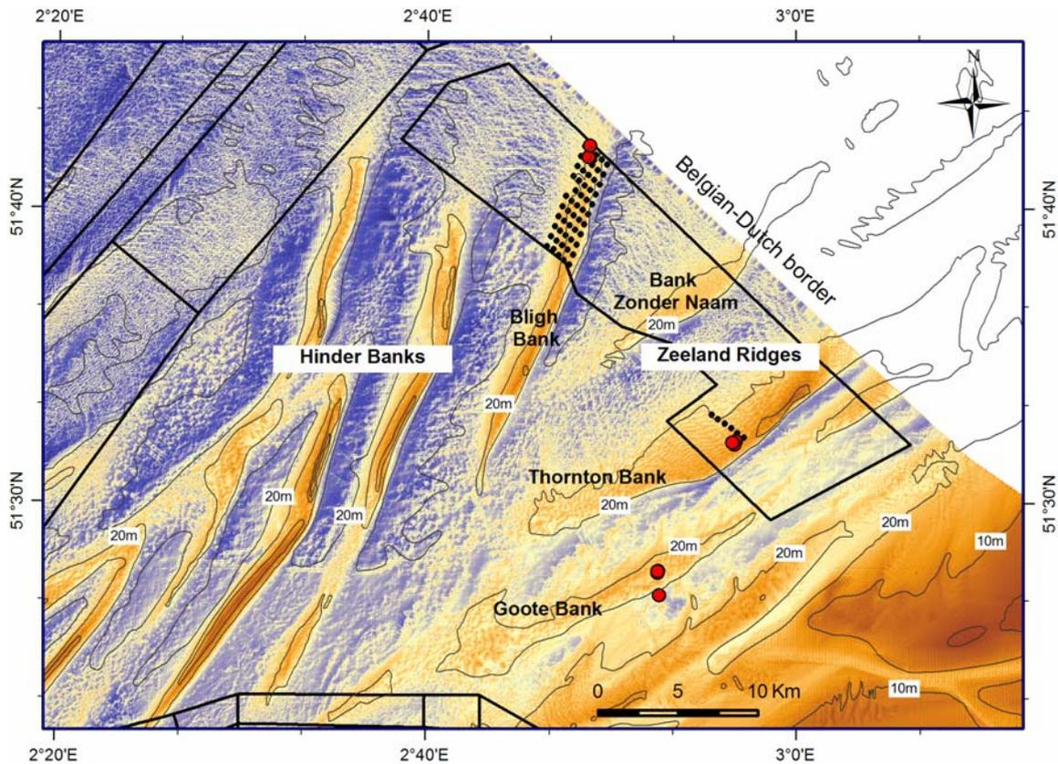
Figure 1: Bathymetry of the Thornton Bank, Bank Zonder Naam, Bligh Bank and Goote Bank. The black dots indicate the position of the windmills, the red dots indicate the position of the turbidity and current measurements.
