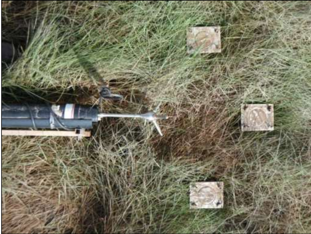
Figure 8: ADCP and sediment covered traps at M1 on August 31 st , 2011 (Photo by C. Skinner, 2011). Note deployment of the ADCs at M1 and M2 side lying in order to sample as close to the bed as possible.
