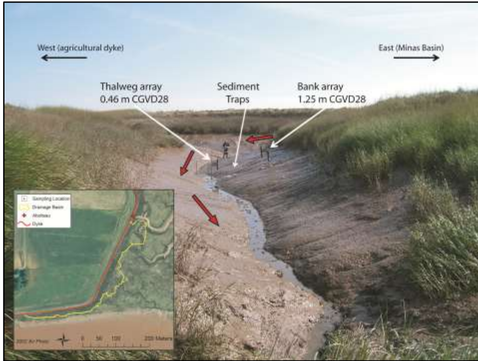
Figure 3: 2009 experimental set-up within end member tidal creek at Starrs Point. Localized drainage basin indicated within the inset.
