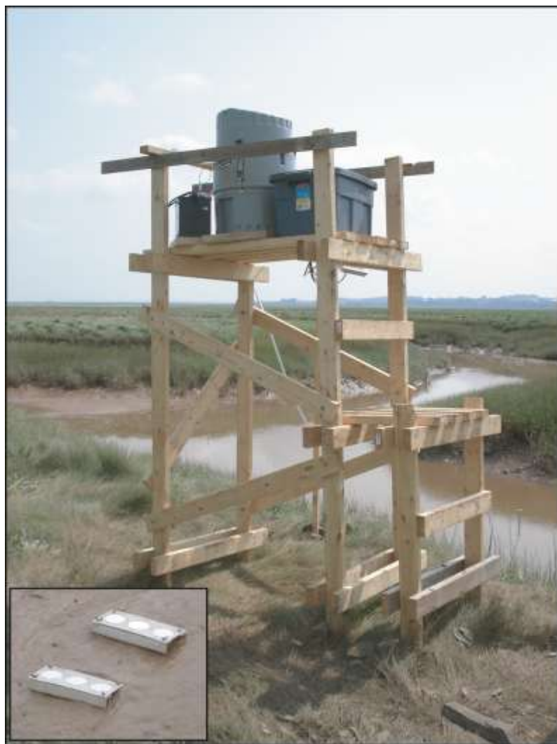
Figure 5: ISCO sampling platform on the high marsh surface adjacent to the tidal creek used in both 2009 and 2011 deployments. Structure was removed during the winter months. Surface mounted sediment traps used in 2009 depicted within the inset.
