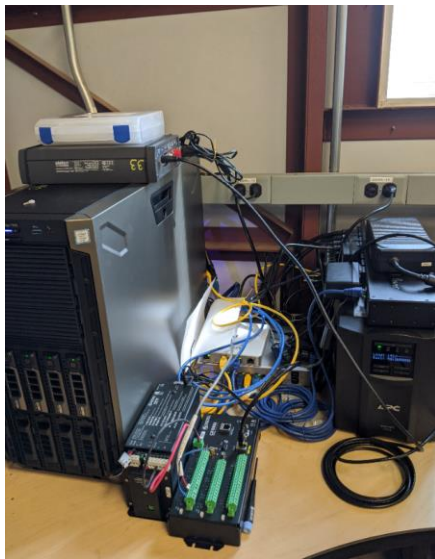
Figure 9. The EchoSense decision subsystem in the NREL lab. The Campbell Scientific Datalogger and the Acoustic detector are connected to the server.
