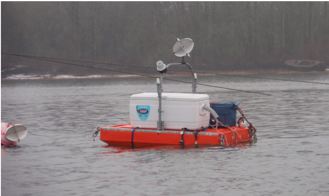
Figure 4.3. A Photograph of the Barge with the Sensor Recording Box and Air Pump Secured Within the White Cooler. Fish cages and blast sensors are deployed off the aft end of the barge. The barge was equipped with low-visibility safety gear and extra line (blue container).
