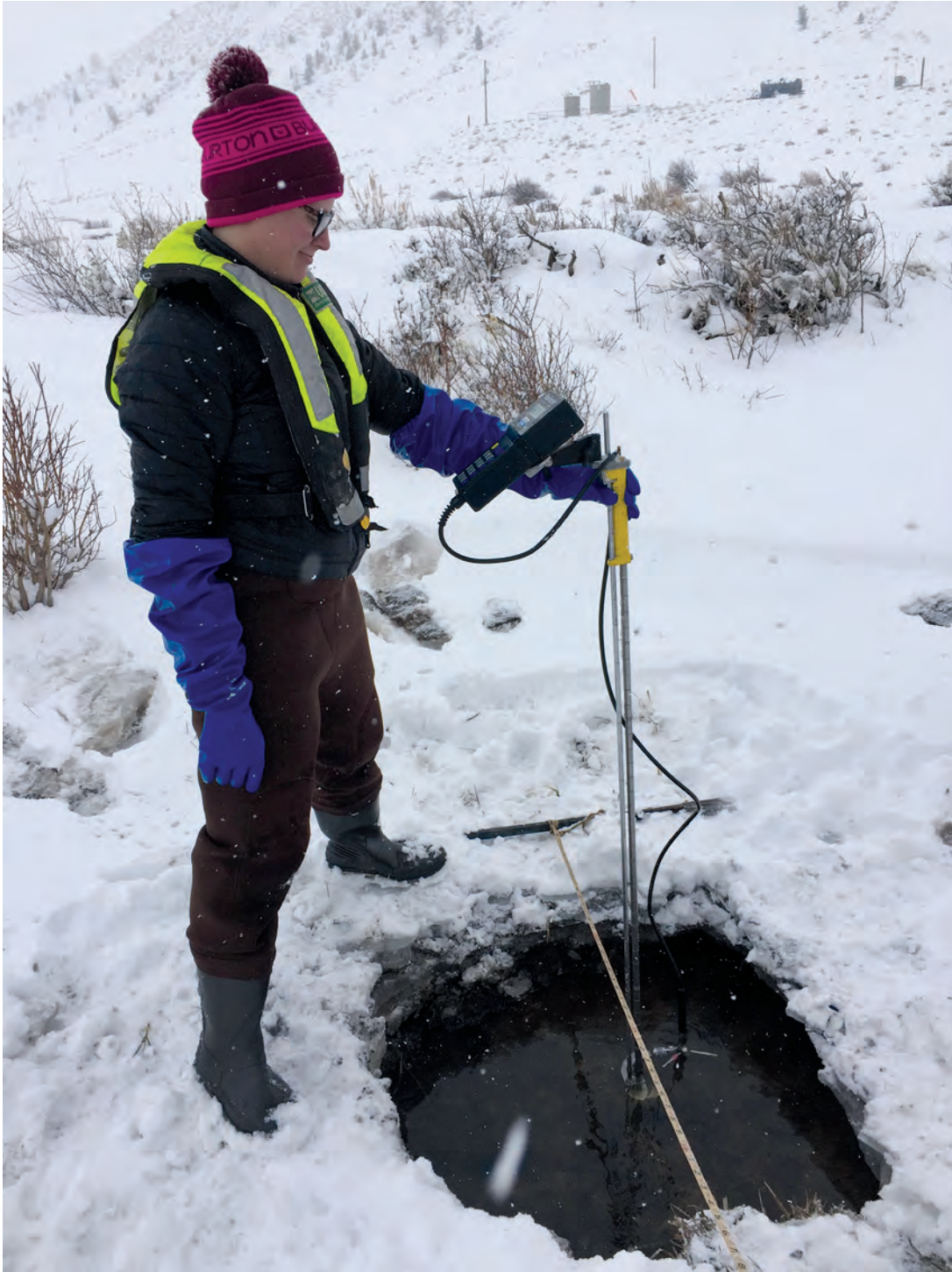
Figure 7. Photograph of a U.S. Geological Survey researcher (associated with the Wyoming-Montana Water Science Center) using survey and Global Positioning System (GPS) equipment to verify streamflow measurements in South Beaver Creek in Wyoming during February 2018. Photograph by Cheryl A. Eddy-Miller, U.S. Geological Survey, 2018.
