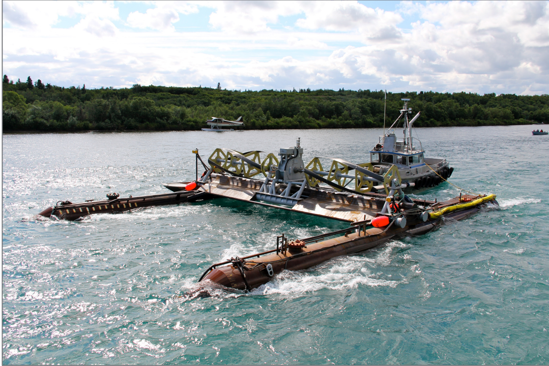
Figure 2.1. Photograph of the ORPC RivGen ® device.
