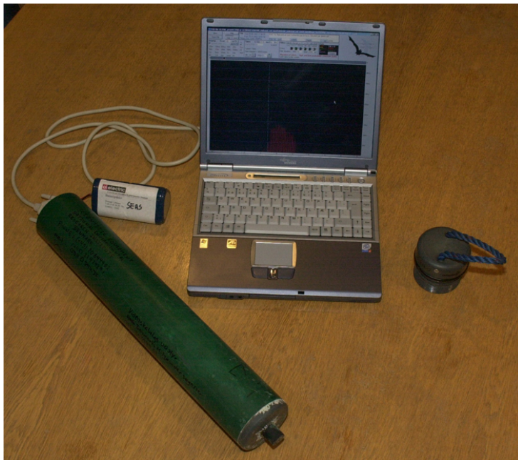
Figure 7. An open T-POD connected to a computer. The hydrophone can be seen as a small attachment in the lower end of the T-POD. A prefabricated 6x D-cell Li-Ion battery pack is seen behind the T-POD.
