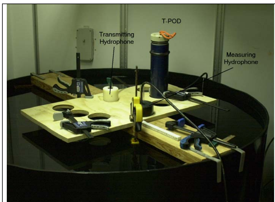
Figure 21. T-POD calibration test tank. One T-POD (out of six possible) is mounted for calibration. Transmitting hydrophone is placed in the centre of the tank. Water depth is approx. 90 cm.
