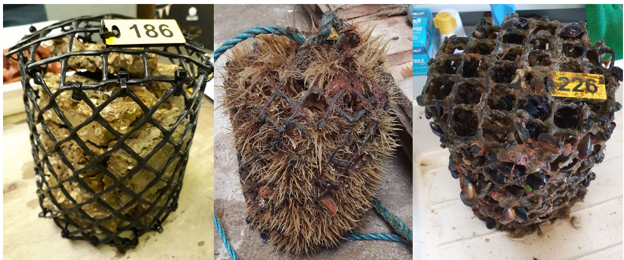
Figure 8: Illustration of the different degrees of biofouling on the baskets with substrates in different locations as they were collected to be counted. A) New Quay; almost no biofouling. B) Tralee; high degree of biofouling. C) Grevelingen; high degree of biofouling by mussels ( Mytilus edulis ) and skeleton shrimps ( Caprellidae ) is visible.
