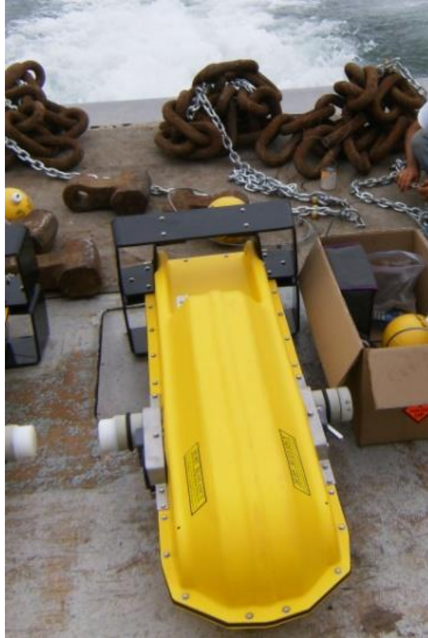
Figure 5. Rigging units for deployment of C-PODs. Mooring chain weights can be seen on the stern of the vessel. Photo courtesy of Colin Buhariwalla.
