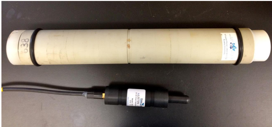
Figure 9. Images of a C-POD (top) and an icListenHF hydrophone (bottom). See Table 4 for specifications.
