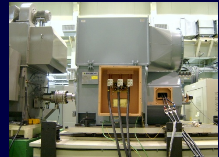
600kW Doubly-fed Induction Generator
