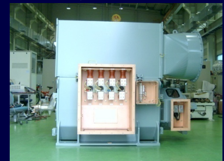
600kW Synchronous Generator
