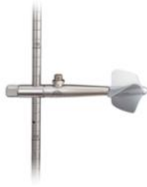
Figure 2-3: Turbine flowmeter (taken from [14]).
