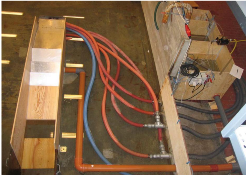
Figure 3-7: SSG overtopping device setup (from [7]).
