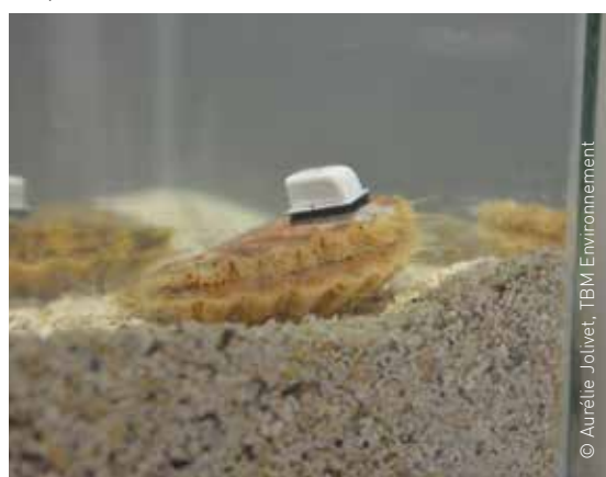
Fig. 43. Accelerometers attached to the great scallops.
