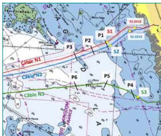
Fig. 9: Positions of the profiles (P1 to P6) and stations (S1 to S3) initially planned for measuring the electromagnetic fields along the Jersey-Cotentin connection comprising the N1, N2 and N3 cables, using the PASSEM tool.
