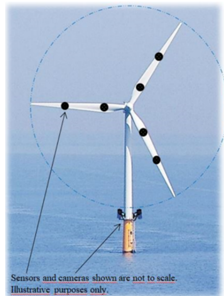
Figure 7 Illustrative representation of the WT-Bird® system with impact detection based on fibre optic vibration sensors and species recognition based on high quality camera images
