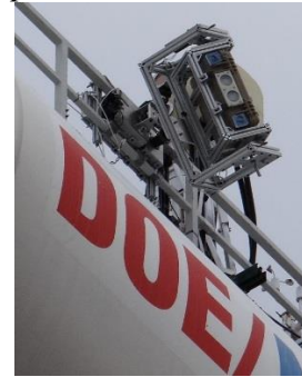
Figure 2.2.3. Pan-and-tilt frame attached to railing on nacelle of Cart 3 turbine at NREL.
