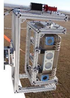
Figure 2.2.2 Pan-and-tilt frame for optics node.
