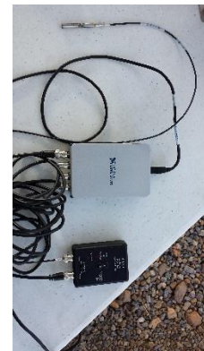
Figure 2.3.2. Integrated bioacoustics node showing the microphone (top), analogue to digital converter (middle), and microphone power module with filter (bottom).
