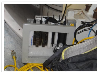
Fig. 2.1.4. Receivers for wireless contact microphones and accelerometers were placed inside the nacelle.
