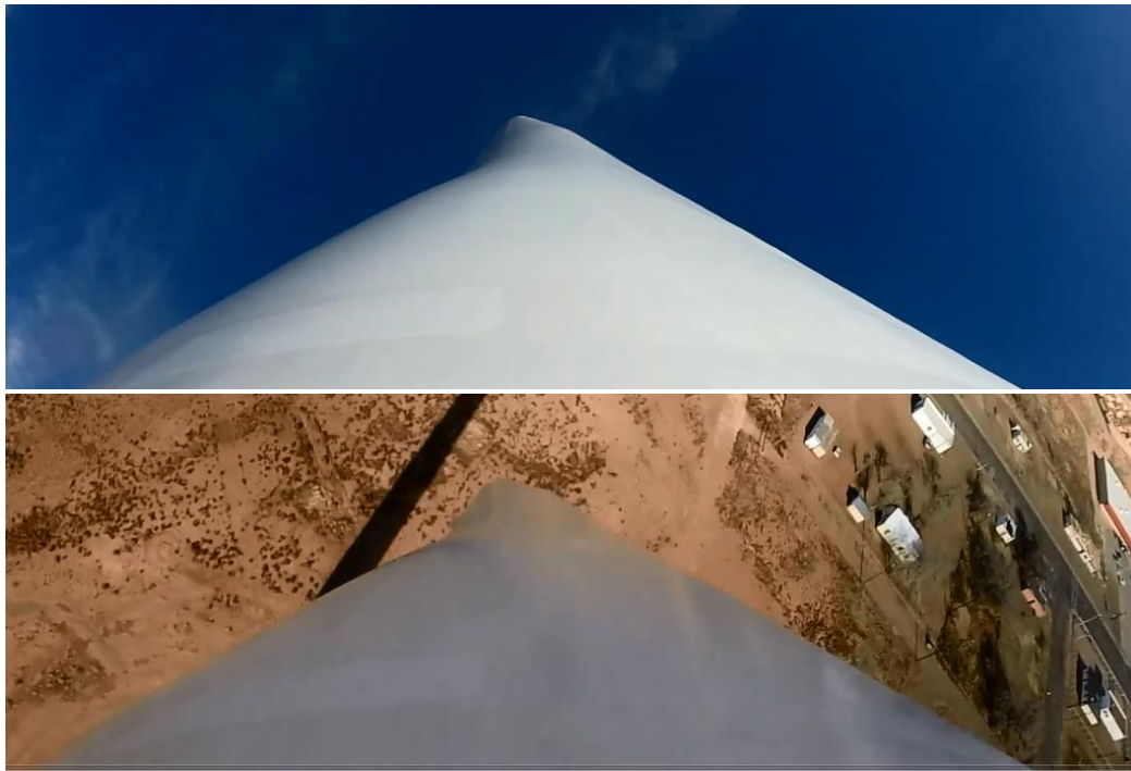
Figure 3.2.8. Views from a GoPro camera mounted at the root of the blade with sky and ground background on the GE turbine at MCC. Placement of cameras on turbine blade is a likely solution to provide the resolution needed for target identification while minimizing the number of cameras needed to cover the entire rotor swept area.
