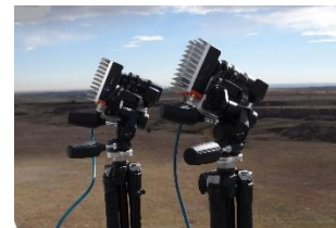
Fig. 2.2.4. Smart cameras with onboard image processing ability.
