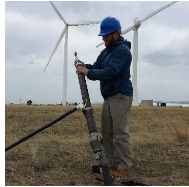
Figure 2.6.1. Compressed air cannon used to create experimental impacts on research turbines.
