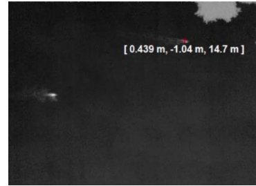
Figure. 3.2.4. Target tracking (50 fps) and distance calculation of a bat. Two bats are in image. Species was either silver-haired, California myotis, or little brown – all were present in audio recordings during image capture.
