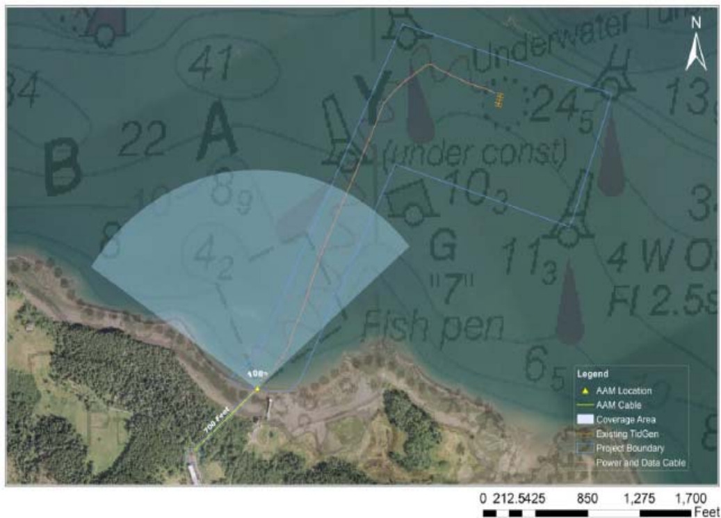
Figure 6: The final location of the system, monitoring region, and the location of the TidGen and original deployment location.
