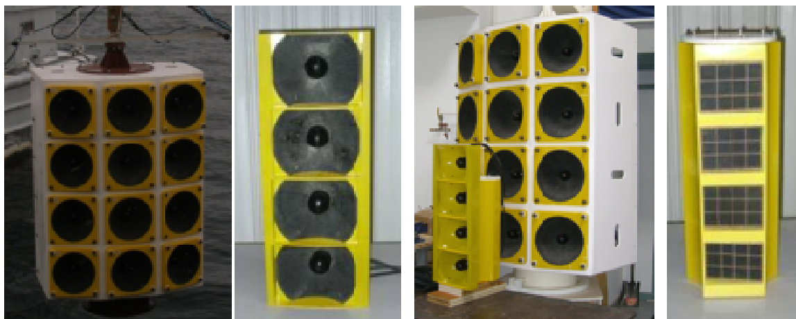
Figure 1: SDSN nodes. On the left is the original production node that has 12 round parabolic reflector transducers. On the left center is the second-generation (G2) node that has 4 rectangular parabolic reflectors transducers. On the right center is a comparison of the size of the current node and G2 node (black foam has not been installed in the G2 node). The new node is roughly 1/8 the size and has the same or better performance. On the right is a mock-up of the G2 node with high frequency rectangular flat plate transducers. This would operate between 90 and 120 kHz and is similar to what was developed for this project.
