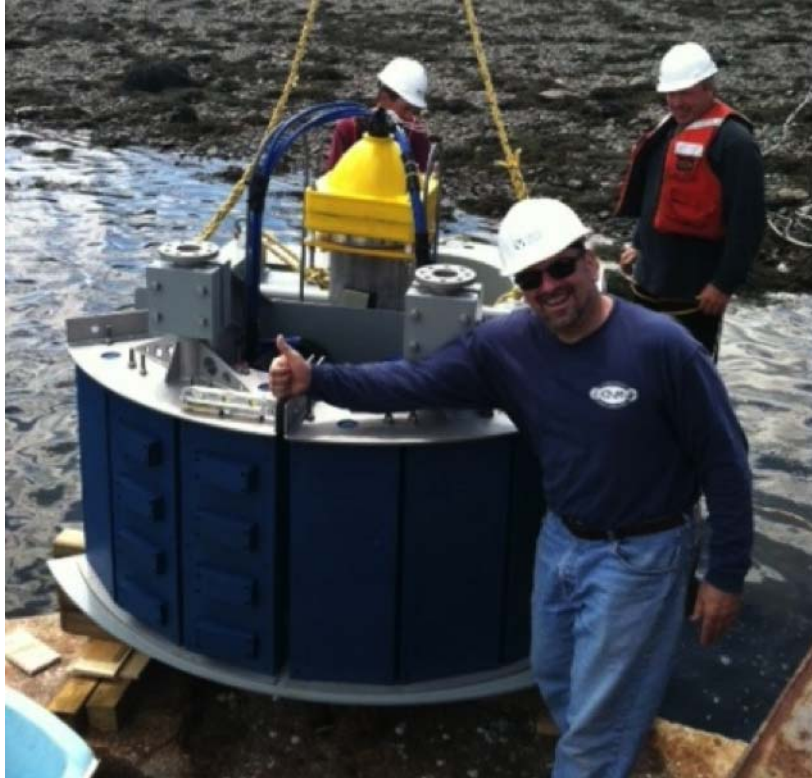
Figure 9: SDSN nodes deployed on leveling blocks at low tide.
