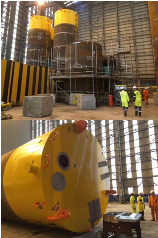
Figure 2.3. Pictures and drawing of suction anchors
