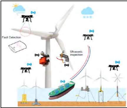
Figure 6-3. FOWT Inspection Drones
