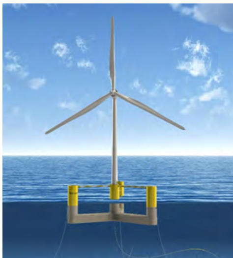
Figure 2-1. Indicative Floating Foundation
