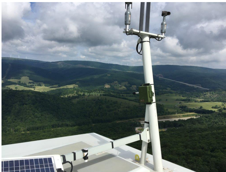
Figure 2-1. Photo of acoustic bat detector (in green box) mounted on the nacelle of Turbine 1 at the New Creek Wind Project (photo from 2017).
