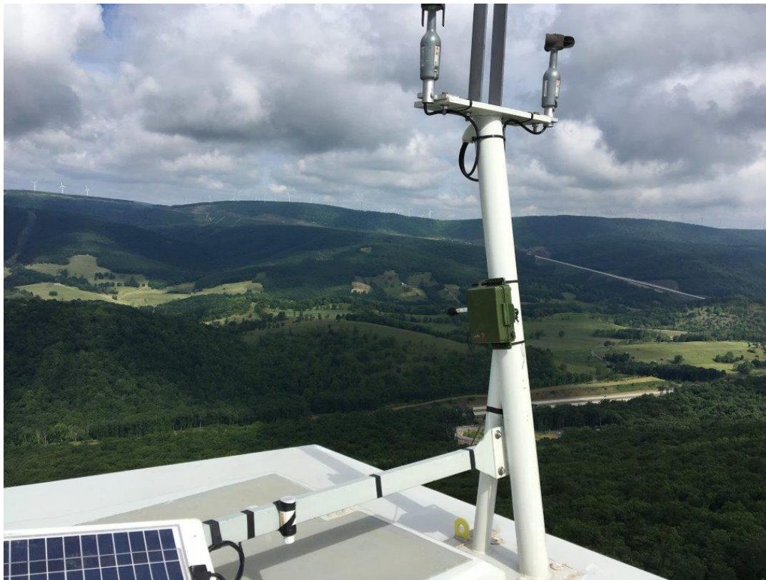
Figure 2-1. Photo of acoustic bat detector (in green box) mounted on the nacelle of Turbine 1 at the New Creek Wind Project, 2017
