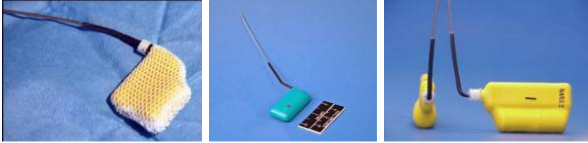
Figure 4-2. Left: PTT prepared with sterile mesh for implantation in Surf Scoter. Center and right: Two antennae configurations of pressure proofed implantable PTTs.
