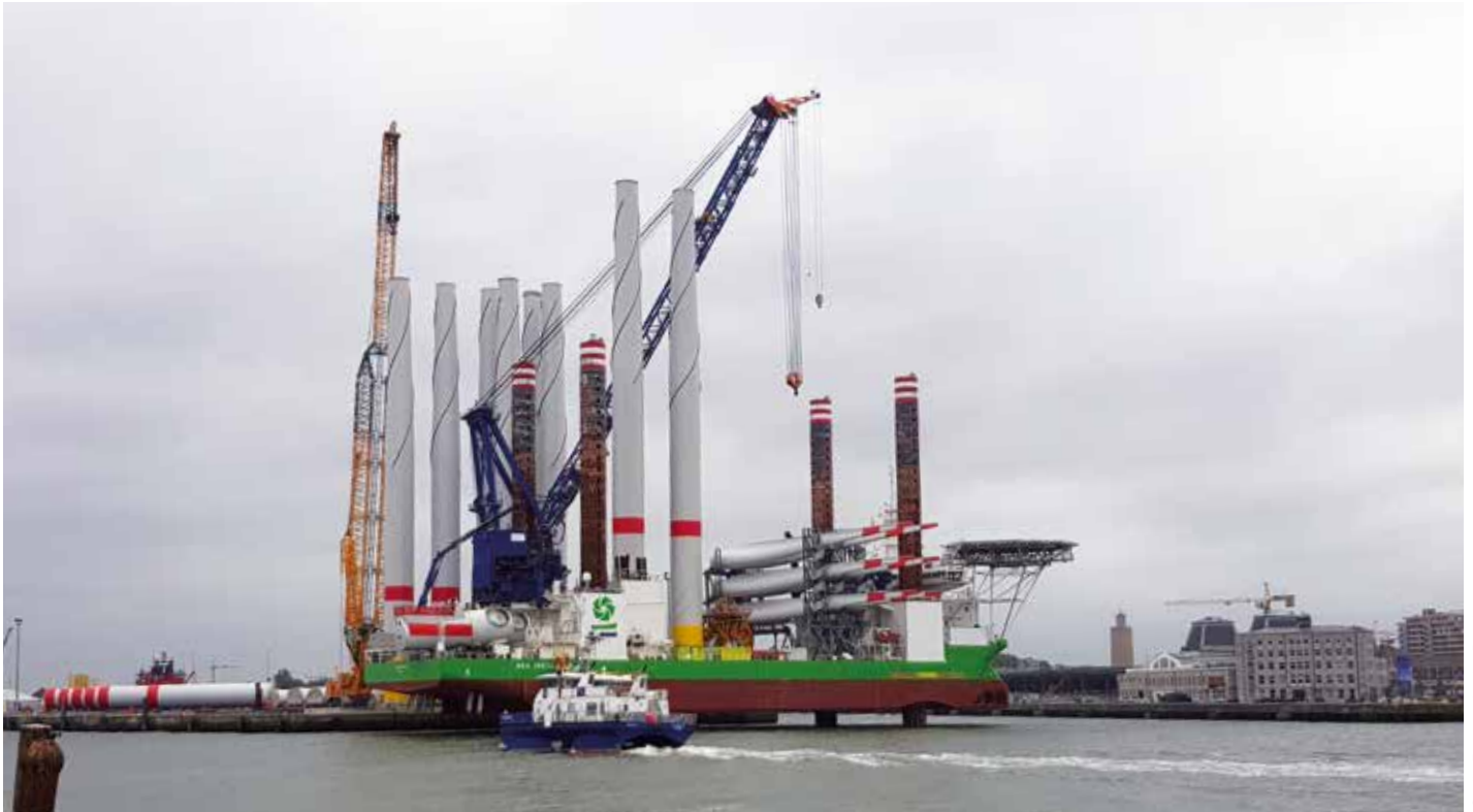
Sea Installer vessel loaded with offshore wind turbine towers and blades in Ostend, Belgium.
