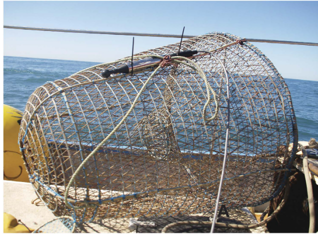
Figure 10. Position of the SMID hydrophone on the cage.
