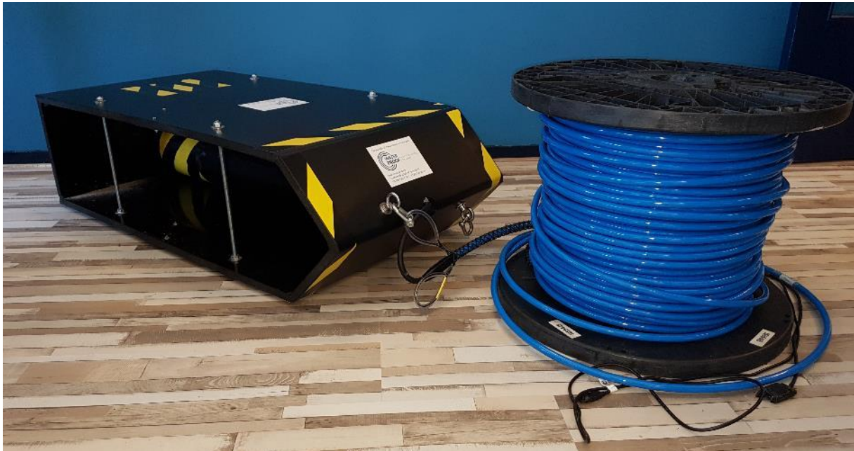
Figure 2.12: Measurement sledge for EMF measurements and video observations (camera system not installed here), with umbilical cable.
